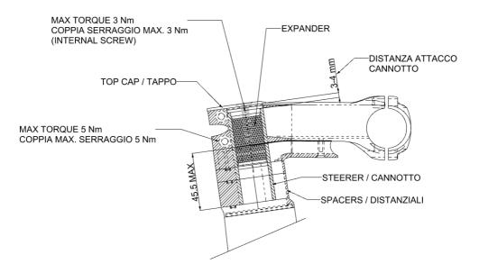
Fig. 5.1: Superbox assembly schema with S-DCR cover system
