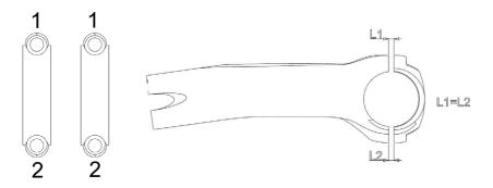
Check the symmetry and equality of all the distances between faceplate and stem body, if necessary. The distance between the faceplate and the attachment body must be the same on the upper and lower part.
